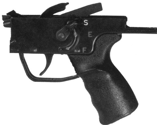
modified HK selective fire trigger housing
