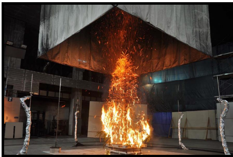
Figure 18 – Burning embers floating down late in test
