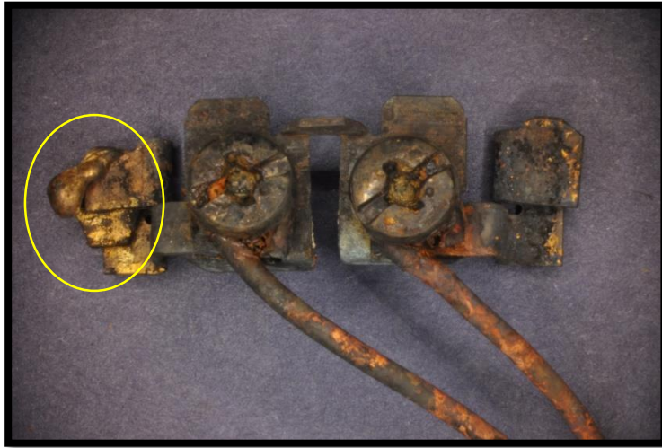
Figure 11 – Plug blade with localized melting
